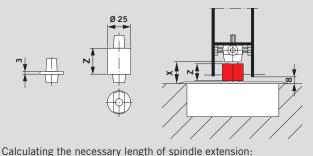
Calculating the necessary length of spindle extension: Extension = X – Floor clearance (normally 8 mm)
